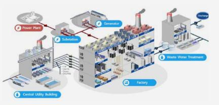
Samsung SDS Intelligent Factory features a monitoring system that analyzes wastewater and emissions components, flow rates, and temperatures and monitors them to prevent any violations of environmental regulations.
