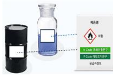
< Attachment of Warning Signs >
